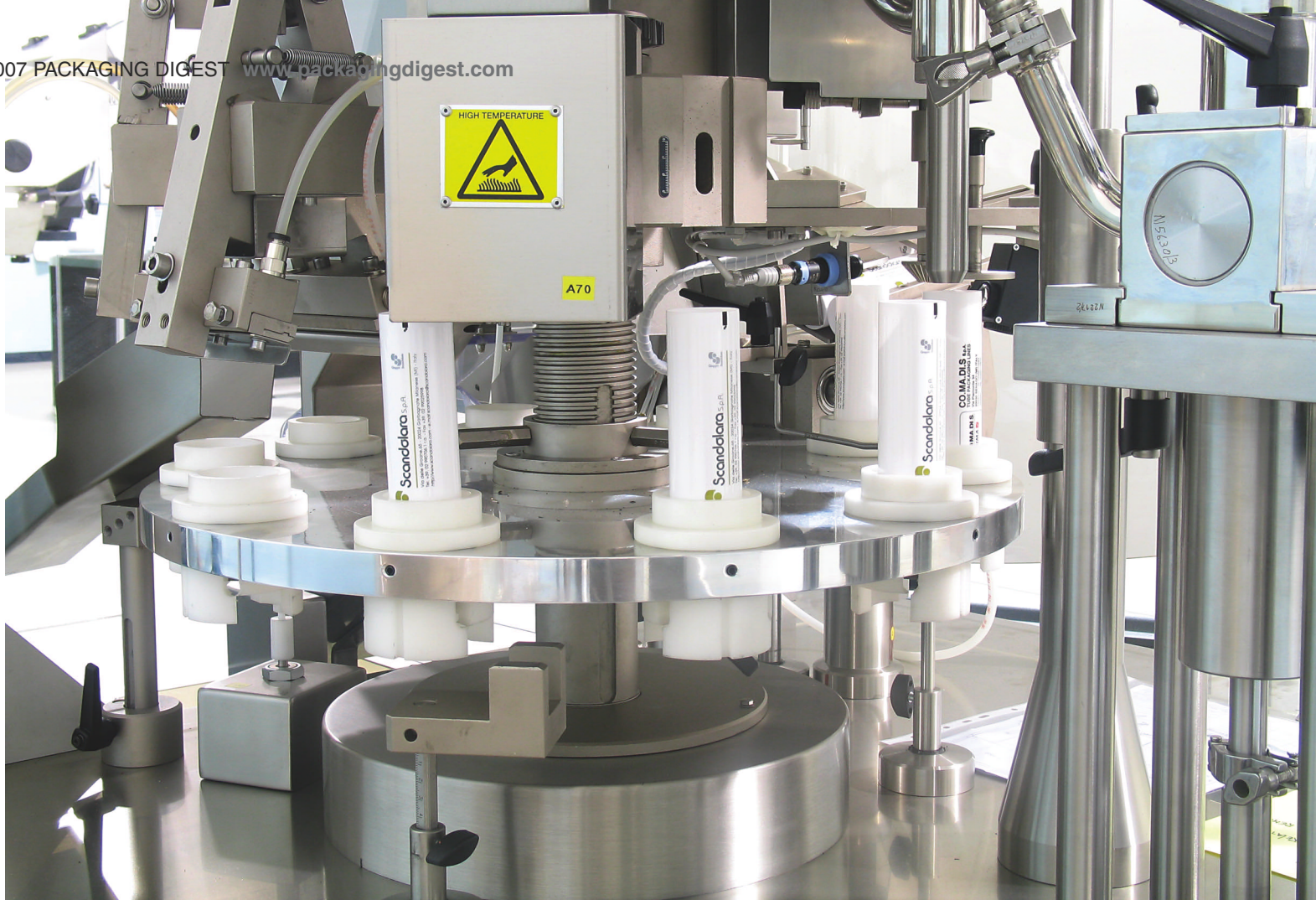
Tubes drop into a 15-position turntable that transports them through filling, sealing and inspection sections.
